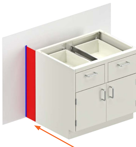
3 Use screws to attach the L-Filler to the base cabinet.
