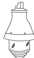
Explosion Proof Light Class 1, Group 1 Available in Incandescent or fluorescent Part # XPL
